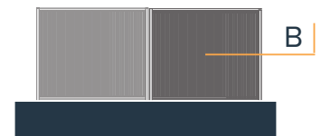
SECTION B 0.95MM POST WITH ADDITIONAL 65X65X2.5MM SHS
